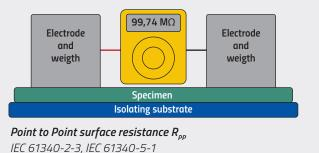
The moisture attraction and formation of an anti-static layer leads to a resistivity of approx. 105  $\Omega$ . As stand-alone additives quats do not reach true conductivity.
