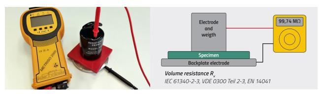
Setup for measuring the surface resistivity:
